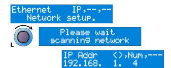
At the end of the scan, which takes a few seconds, the display updates with an IP address as shown above. The Default IP Address is 192.168.1.1.
